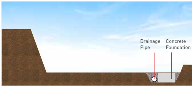
Foundation of the reinforced wall
